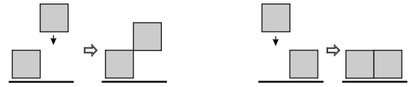
FIG. 2. Updating rules for the asymmetric NNN ballistic deposition defined in Eq. (2a).
